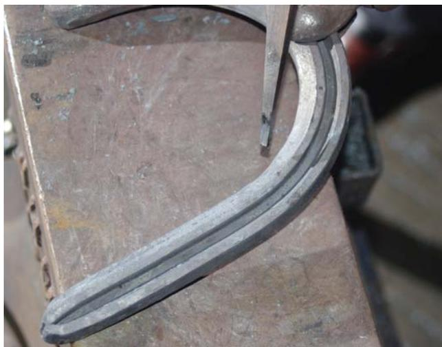
**6.10** At this point there is a marked kink, or shoulder, in the metal, just away from the toe bend (see pointer). This will need to be straightened, and in doing so the toe will open out slightly.
