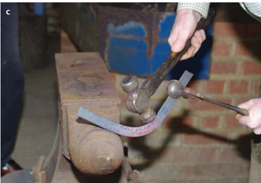
**6.6** Forming the toe bend. An even heat needs to be taken centred on the middle of the bar, and extending outwards to involve half the bar.
