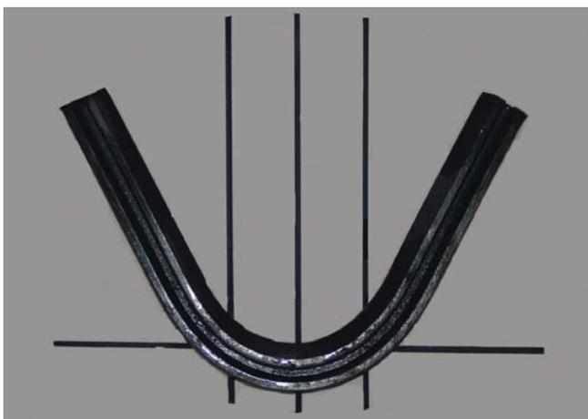
**6.8** Assess the toe bend to ensure it is symmetrical about the centre of the bar.
