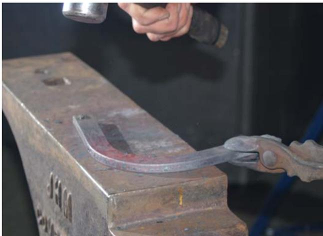
**6.7** Level the shoe to remove any buckling, before proceeding.
